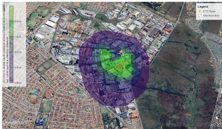
Figure 6-18: Simulated metal annual average incremental concentrations for the proposed plant-New Plant Standard Scenario (assessment criteria – 0.02 \mu\text{g}/\text{m}^3 ).
