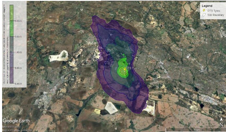
Figure 6-17: Simulated metal hourly average incremental concentrations for the proposed plant-New Plant Standard Scenario (assessment criteria – 0.2 \mu\text{g}/\text{m}^3 ).
