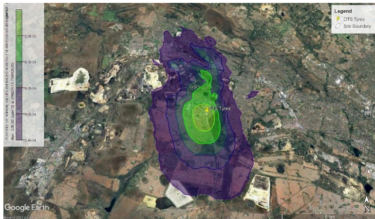
Figure 6-2: Simulated PM 10 annual average incremental concentrations for the proposed plant-New Plant Standard Scenario (assessment criteria – 40 µg/m 3 ).
